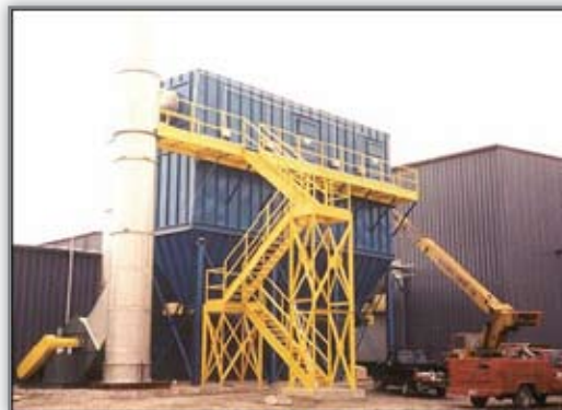
960 Bag Pulse Jet Collector with 15,700 Ft 2 of Cloth Mold Fume Line - High Density Polyester at 110°F
