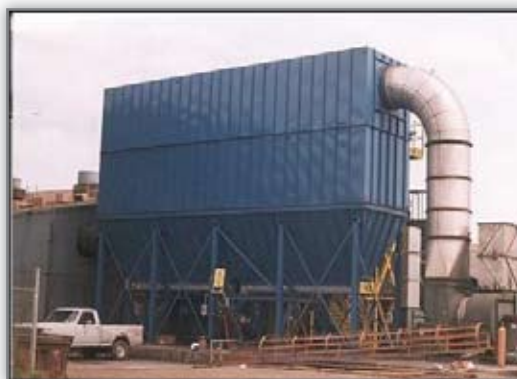
1224 Bag Pulse Jet Collector with 20,000 Ft 2 of Cloth Foundry Process Gas - High Density Polyester at 220°F
